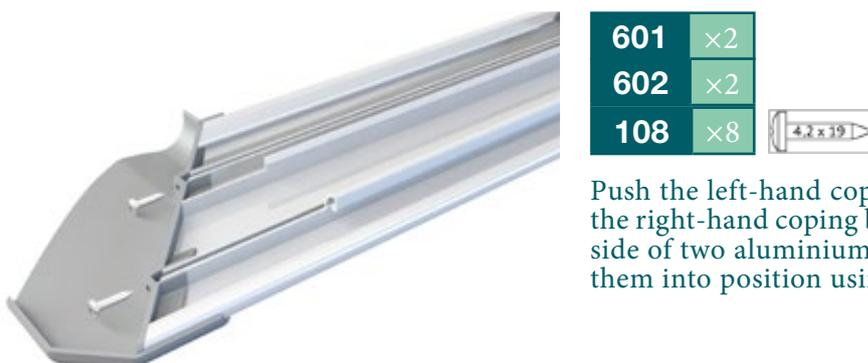
Push the left-hand coping blocking plug (601) and the right-hand coping blocking plug (602) into each side of two aluminium copings (212-A), and screw them into position using 2 screws (108) per plug.
