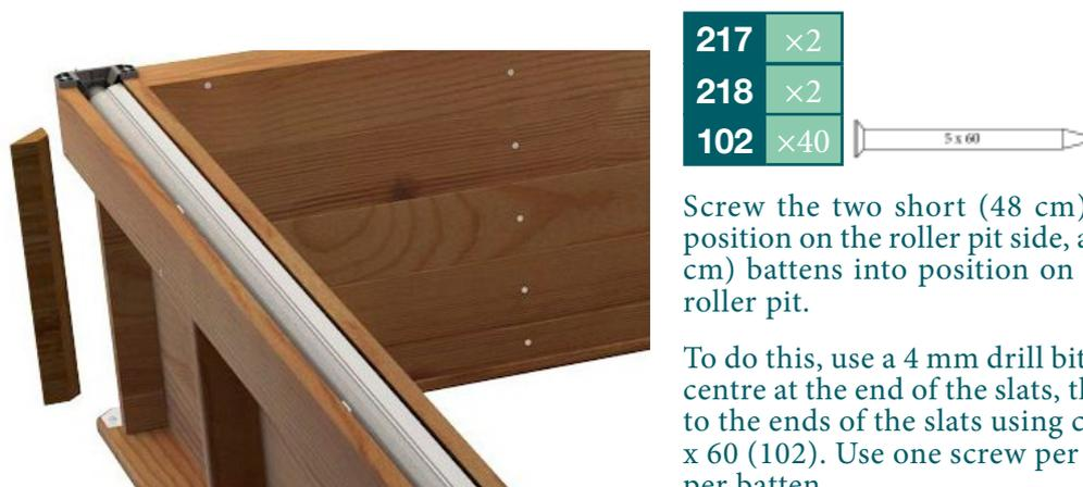
Screw the two short (48 cm) corner battens into position on the roller pit side, and the two long (60.7 cm) battens into position on the side opposite the roller pit.
